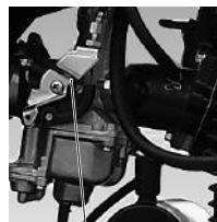
Idle bolt (carburator)
